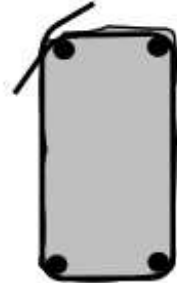
Figure 2.6 – Comparison of Anchorage between 90° and 135° bends
