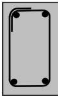
Figure 2.6 – Comparison of Anchorage between 90° and 135° bends
